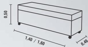
ASSENTO: ESPUMA SOFT D28 / 6CM DE ALTURA / RECOBERTA COM MANTA ACRÍLICA PARA MAIOR CONFORTO
